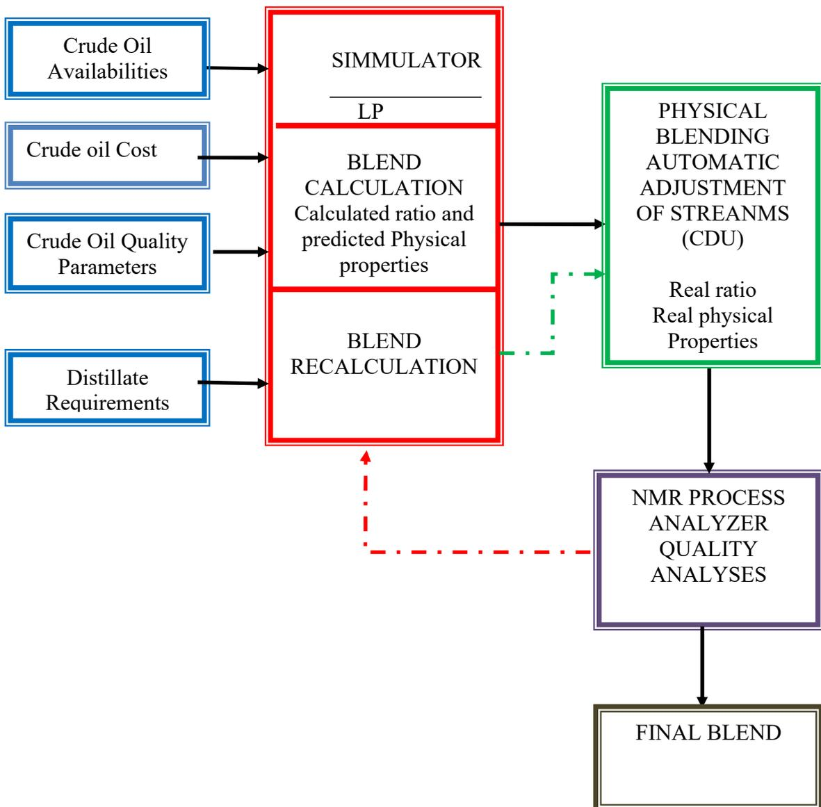
Figure 7: Dynamic Process of Mixing, Continuous Blend Analyses, Simulation Model Adjustment and Process Control.
