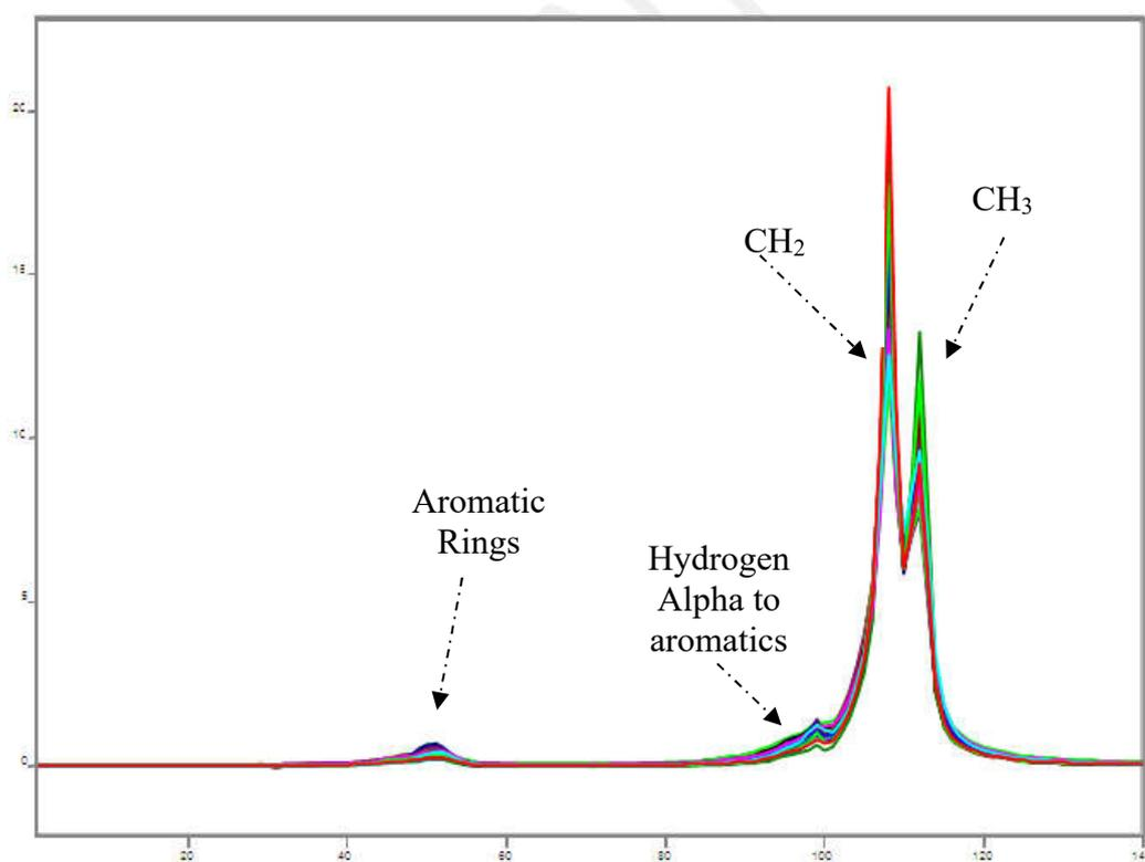
Figure 2: Typical NMR Spectra of Crude Oils:
