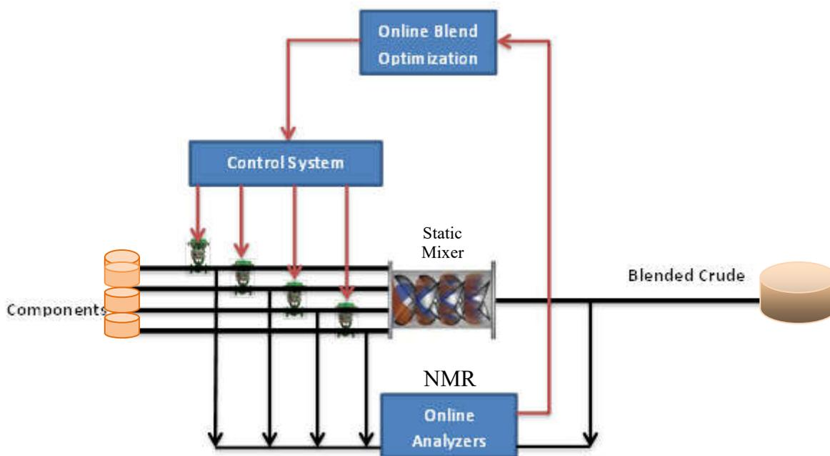
Figure 6: Set Up Of A Blending Station With Incorporated next generation NMR Process Analyzer, Simulation Modeling and Blending Control. (Components can be high and low quality crude oils, diluents and/or gasses (NLG)).
