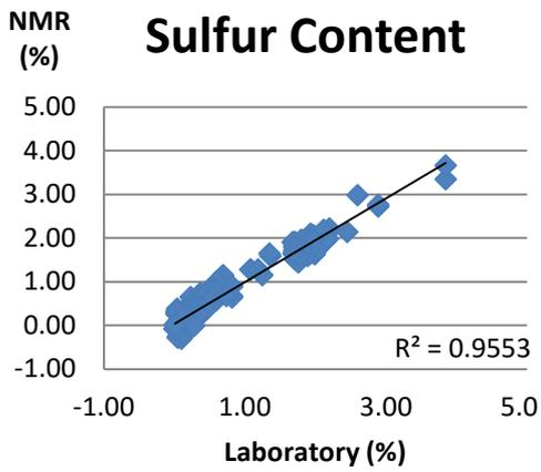
Figures 3: Correlation between NMR Results and traditional Laboratory Measurements.
