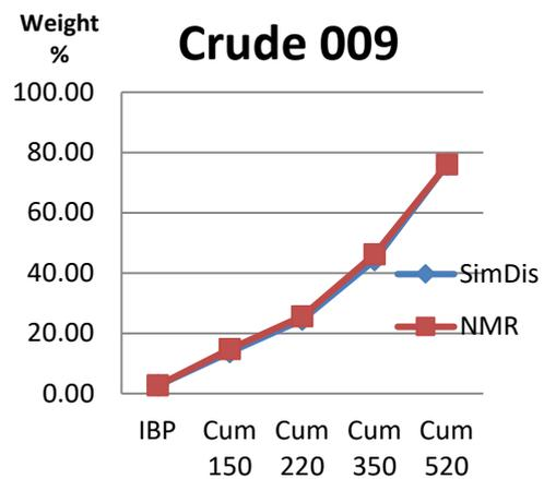
Figures 5: Overlapping NMR and SimDis Predicted Distillation Curves.
